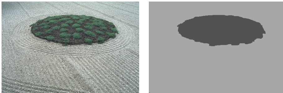
Figure 2: The figure shows the input image and a global minimizer of (2) for parameters \lambda_1 = \lambda_2 = 0.0001 , \mu = 1 and \nu = 0.1 . The optimal foreground and background colors were found as c_f^* = 81 and c_b^* = 167 .
