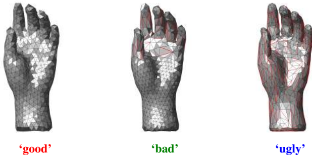
Figure 7: Convergence of our optimization problem depending on the quality of the mesh (top; shown is MfO energy). Red: a ‘good’ mesh (bottom left) obtained with isotropic remeshing and containing no obtuse triangles results in all positive cotangent weights, which leads to fast convergence. Green: a ‘bad’ mesh (bottom center) contains few obtuse triangles, resulting in some negative weights (respective edges are shown in red), leading to a slower convergence. Blue: an ‘ugly’ mesh (bottom right) containing many obtuse triangles breaks the convergence.
