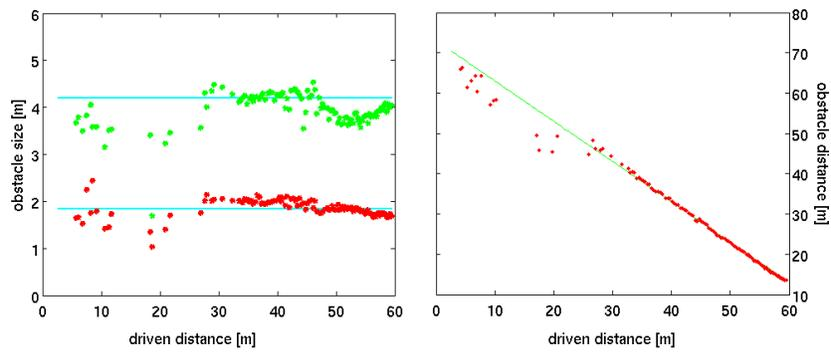
**Fig. 5. Distance and obstacle size estimation for the example with one obstacle (ground truth: 4.19 m  $\times$  1.83 m) in Figure 1.**
