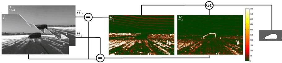
**Fig. 2. Motion-compensated difference images.** From left to right: original gray value input images and difference images for foreground ( $E_f$ ) and background ( $E_b$ ) based on the quadratic difference between the motion-compensated image  $I_{t-1}$  and image  $I_t$  after the last iteration. The camera translation was 1.9 m.  $H_f$  and  $H_b$  denote foreground and background motion.
