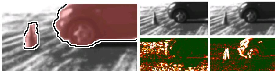
**Fig. 3. Closeup of segmentation for an obstacle in 17 m distance.** The middle image shows the warped foreground with the foreground energy. The right image shows the warped ground plane and according energy. Color warmth denotes higher gray value difference compared to the current image. Notice the correct segmentation across the shadow boundary and the incorrect segmentation of the traffic cone due to occlusion.
