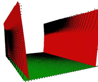
Fig. 1. Birds-eye view of a data set and its planar approximation obtained with the standard EM-based clustering approach. The angle between the normals of the two planes belonging to the parallel walls is 17.2 degrees.
