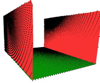
Fig. 3. Model obtained by our hierarchical EM. Compared to the model shown in Figure 1 the angle between the normals corresponding to the two parallel walls is 1.9 degrees.
