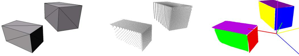
Fig. 8. Simulated scene with more than 3 main directions (left), simulated 3D-scan (center), and resulting planes and main directions (right)
