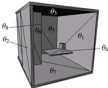
Fig. 6. Simulated 3d scene used to evaluate the quality of the resulting maps. On top of the horizontal plane is a small cube that introduces errors in the plane extraction.
