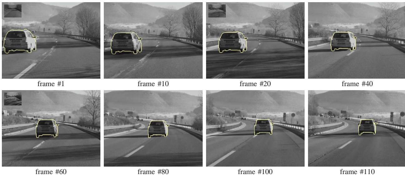
Fig. 10. Stable tracking of deforming silhouettes. The tracking performance is quite robust to changing lighting conditions (caused by shadows and varying shutter times).
