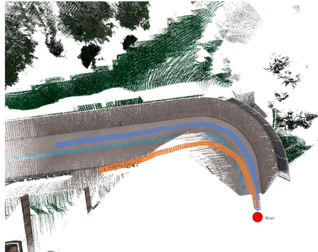
Fig. 10: **Path visualization on a trajectory in the training set with noise level of 10%.** The blue path belongs to the model trained with *Our Method*, while the orange path represents the *Supervised RGB* model. The red dot marks the starting position. *Our Method* is able to keep the lane despite added noise, while *Supervised RGB* leaves the lane shortly after the start and is not able to recover.
