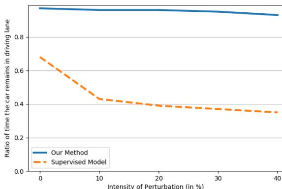
Fig. 9: **Avg. ratio on lane for different levels of perturbation on the training trajectories.** The performance of both the supervised RGB model (orange) and Our method (blue) decreases with higher intensity of perturbations, but the descent is more dramatic for the supervised model.
