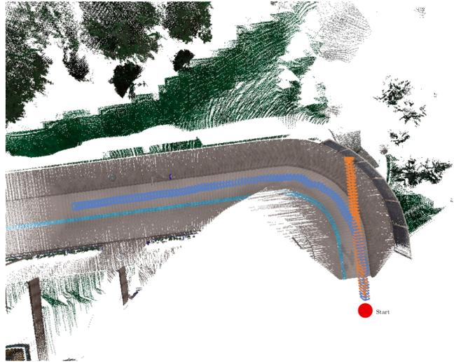
Fig. 8: **Path visualization.** The red dot marks the starting position. *Out method* (blue) was trained using multiple generated trajectories and is able to follow the curve. Meanwhile, the *Single Trajectory* (orange) model was trained using only the single reference trajectory and drives straight into the barrier.
