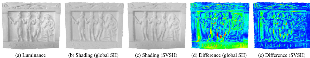
Figure 18. Estimated illumination of Relief dataset: the differences between input luminance (a) and estimated shading (b) and (c) are less for SVSH (e) than for global SH (d), meaning a better approximation of the illumination.
