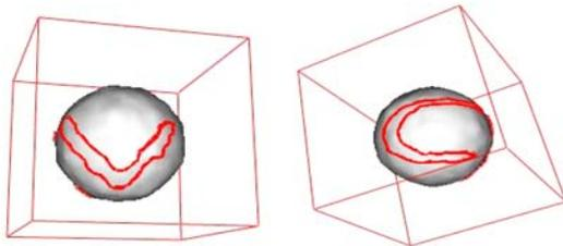
**Fig. 11** The reconstructed shape and partitioning curve between regions with different albedo for the synthesized data in Fig. 10. The two images show the final shape result of the proposed algorithm together with the red segmenting curve. The red straight lines show the coordinate frame for the spheres
