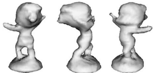
Fig. 4 Final shape estimated using the algorithm (Jin et al. 2004a) with a combination of one positive light and one negative light. The algorithm reconstructs the 3D object more accurately (compared with Fig. 3), nevertheless the lighting configuration if not physically plausible
