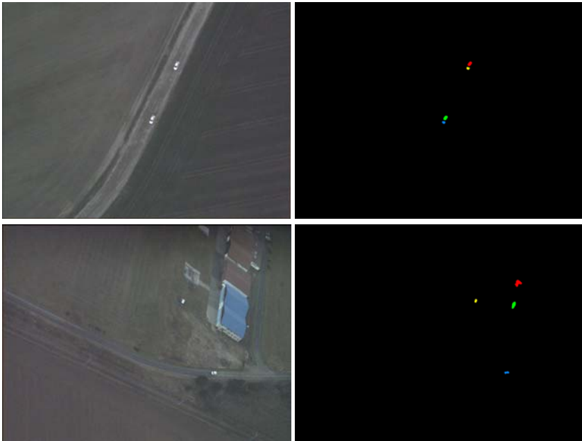
Fig. 5. Object detection results using only color information. Left column: input images. Right column: Detection results presented as colored version of the segmentation result u . Each color represents a label for a pixel.
