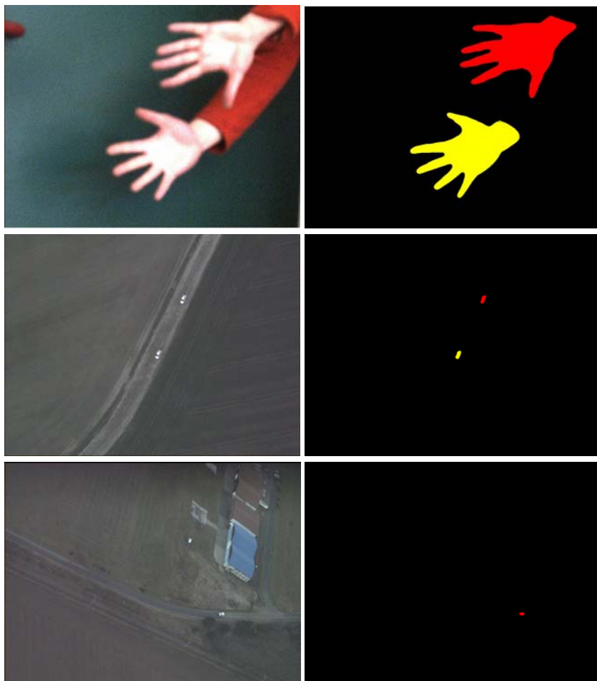
Fig. 4. Object detection results using shape and color information. Left column: input images. Right column: Detection results presented as colored version of the segmentation result u . Each color represents a label for a pixel.
