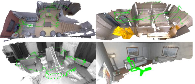
TANDEM is a real-time tracking and dense mapping framework based on dense direct tracking and Deep Multi-view Stereo.
